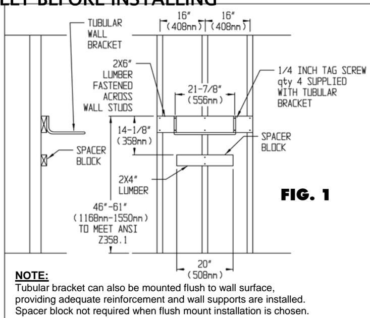
**Caution:** The Eyewash SE-4000 weighs approximately 185 lbs. When filled with 21 gallons of water.
